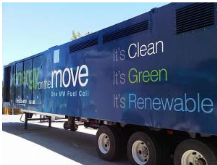
1MW CLEARgen™ fuel cell system
